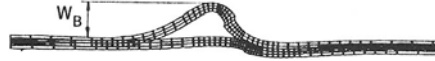
Figure 15. Localization of the axial thermal strains by formation of a bulge shows a typical result of such a 2D finite element analysis.
